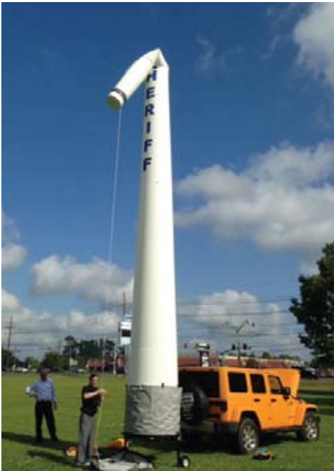
An inflatable tower, powered by a standard automobile outlet, can raise an antenna to further enhance radio communication.
